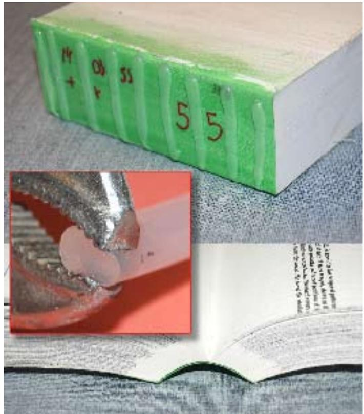
Top: Sample textblock with beads of hotmelt glue added using a standard glue gun. Bottom: The same sample opened. Inset: A pair of pliers show the compressibility of a standard stick of hotmelt glue. When released the glue will slowly return to its original shape.
