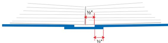
The distance between the corners of the spine is now zero. The corner of the spine has moved in 1/2" relative to the edge of the case spine. The case spine has moved out 1/2" relative to the textblock spine for a total of 1" of movement one side and 2" of movement for both sides.
