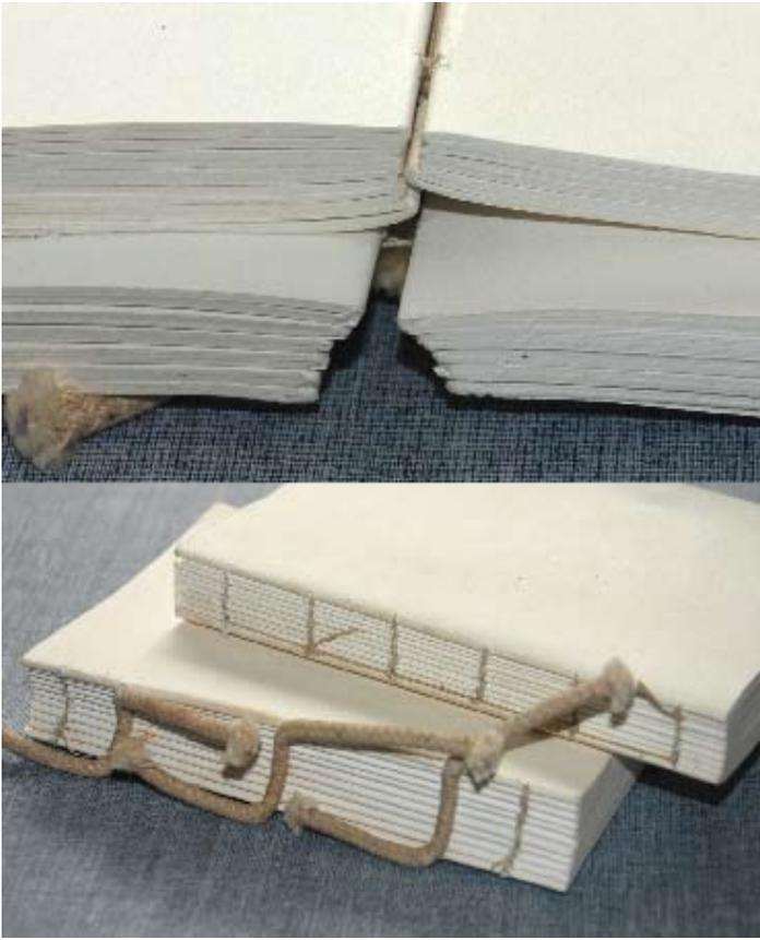
**Sewing and pivot lines** - the two samples above show the effects of sewing on the pivot line. The sample sewn with a chain stitch has a pivot line relatively close to the line of stitching. The sample sewn on cords (actually, clothesline) has a pivot line well removed from the stitching causing a significant spread at the line of stitching when the book is opened flat. This textblock will require significant spine control to prevent it from opening flat and pulling the signatures apart
