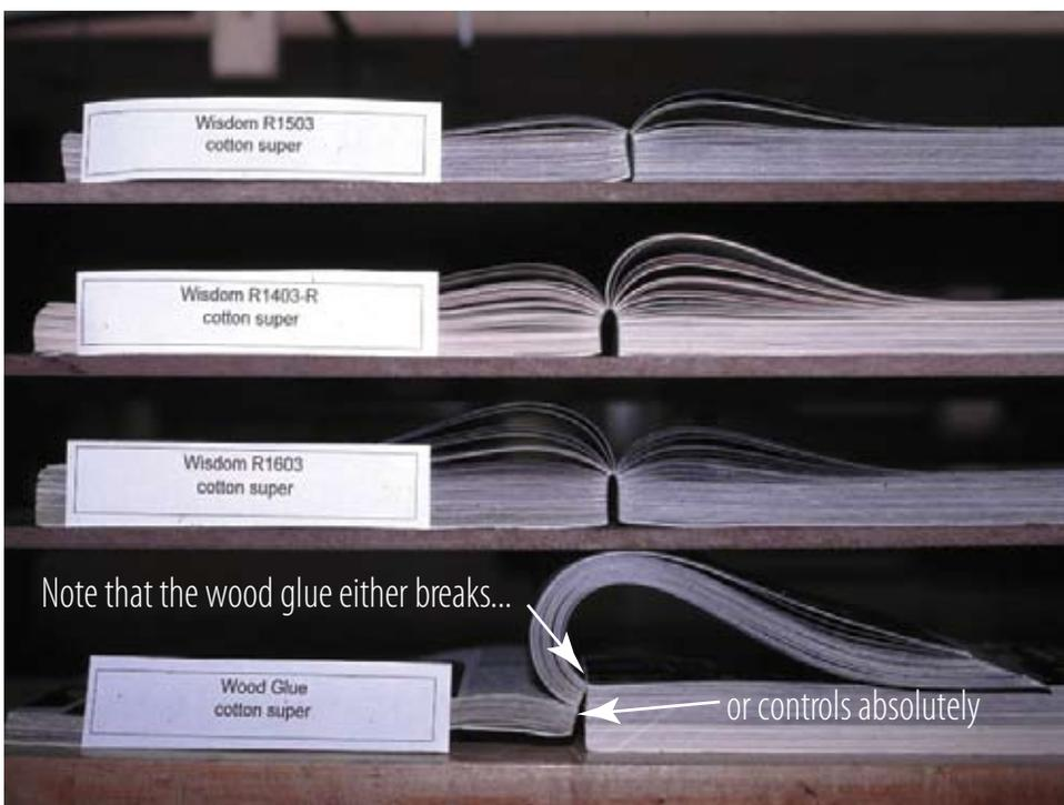
Four samples with the same type of paper, fan-glued with four different glues and lined with a single cloth liner.
