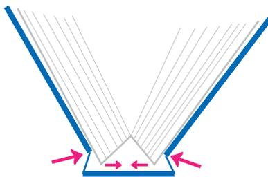
As it opens the two corners of the textblock move toward each other. The joint areas move freely away from the textblock as the boards move with the textblock.
