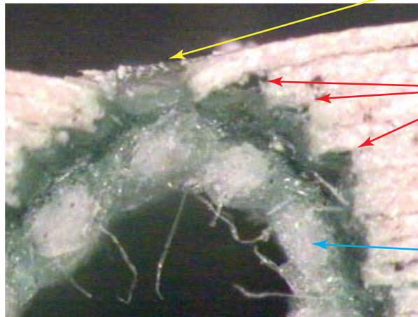
The bond between the opening pages has broken, and the glue line has spread to expand to the arc required by the tight radius.
