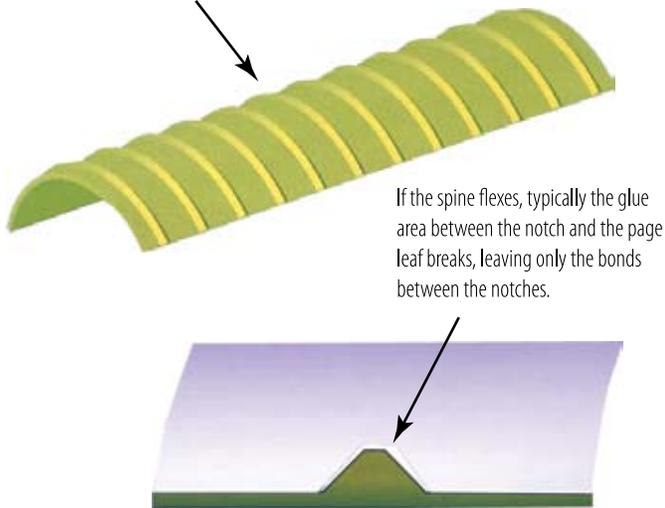
If the spine flexes, typically the glue area between the notch and the page leaf breaks, leaving only the bonds between the notches.
