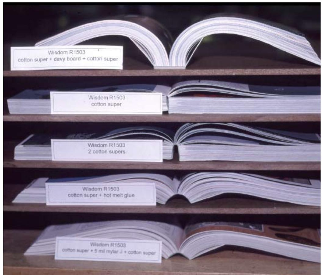
The effects of different linings on spine control - The samples above are all glued with the same PVA but lined differently.
