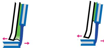
In a traditional tight joint stress concentrates as a peeling stress at the fore-edge of the glue joint. This relationship is maintained through the full opening of the book with the case pulling out and the corner of the textblock pulling in.
